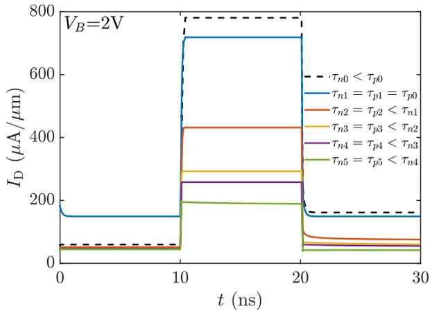
Fig. 8. Time dependent simulations for different carrier lifetimes at  $V_B=2V$ . The dashed waveform corresponds to the carrier lifetimes used in this work.
