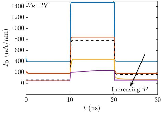
Fig. 7. Impact of the Okuto model parameter ‘b’ on the switching characteristics.
