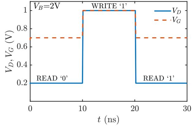
Fig. 4.  $V_G$  and  $V_D$  waveform for switching sequence comprised of READ ‘0’ → WRITE ‘1’ → READ ‘1’. The boost voltage is constant throughout at  $V_B=2V$ .
