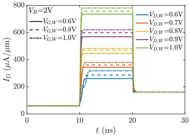
Fig. 9. Switching characteristics at  $V_B=2V$  for different values of drain and gate voltages used for writing.
