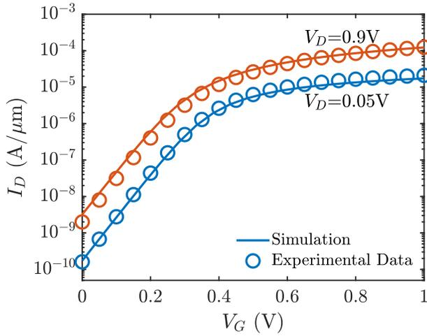
Fig. 2. Calibration of the MOSFET transfer characteristics.
