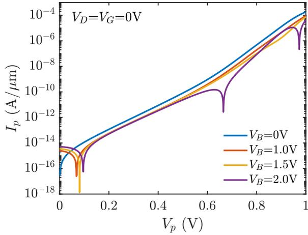
Fig. 3. Base current vs base-emitter voltage ( $I_p$ - $V_p$ ) characteristics of the vertical bipolar transistor at different boost voltages ( $V_B$ ) with  $V_G=V_D=0V$ . Here the subscript ‘ $p$ ’ refers to the floating  $p$ -well region.
