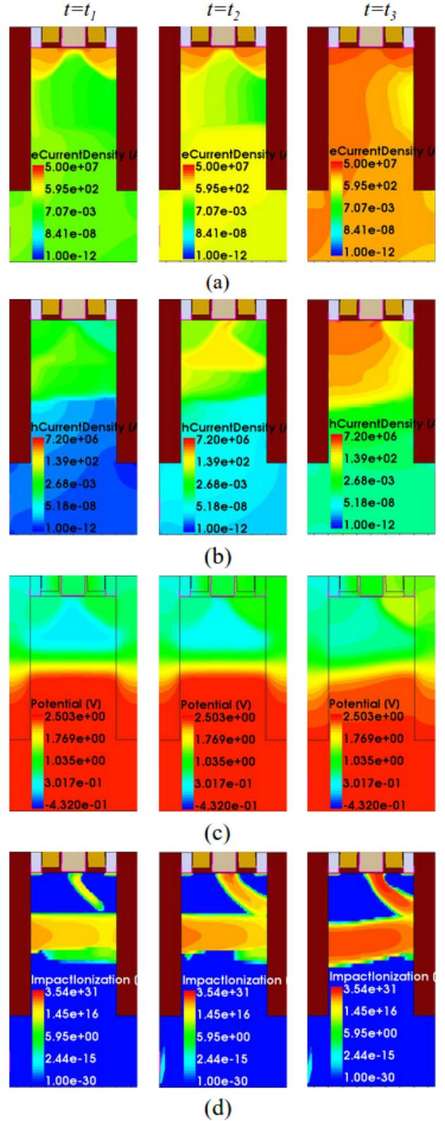
Fig. 6. Temporal snapshots of 2D distributions of (a) electron current density (b) hole current density (c) Electrostatic potential and (d) Impact ionization during the switching.  $V_B=2\text{V}$ . The three time instants ( $t_1$ ,  $t_2$ ,  $t_3$ ) are marked in Fig. 5.
