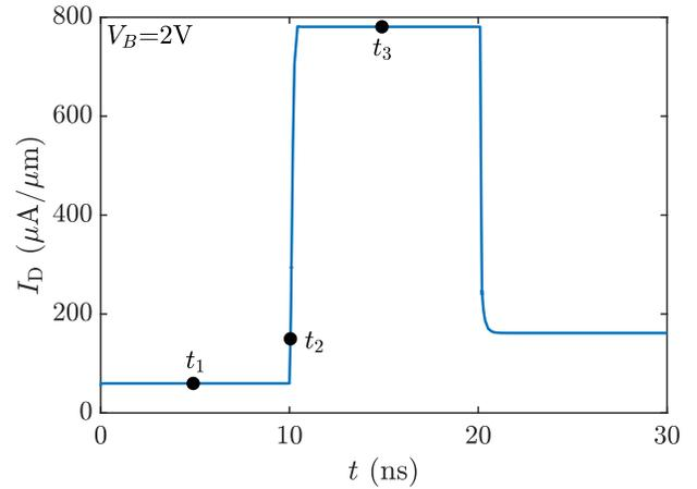
Fig. 5. Switching profile of the 1T-SRAM cell consisting of the READ ‘0’, WRITE ‘1’, and READ ‘1’ operations.
