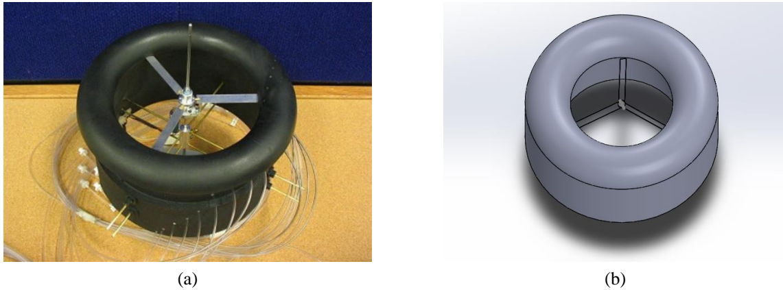
Fig. 15 (a) Experimental system by Pereira [7] compared with (b) CAD representation of shrouded rotor.
