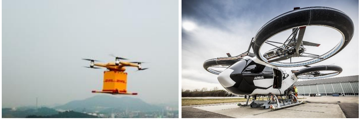
Fig. 1 (a) DHL Last Mile Parcel Delivery Drone and (b) Airbus eVTOL concept.
