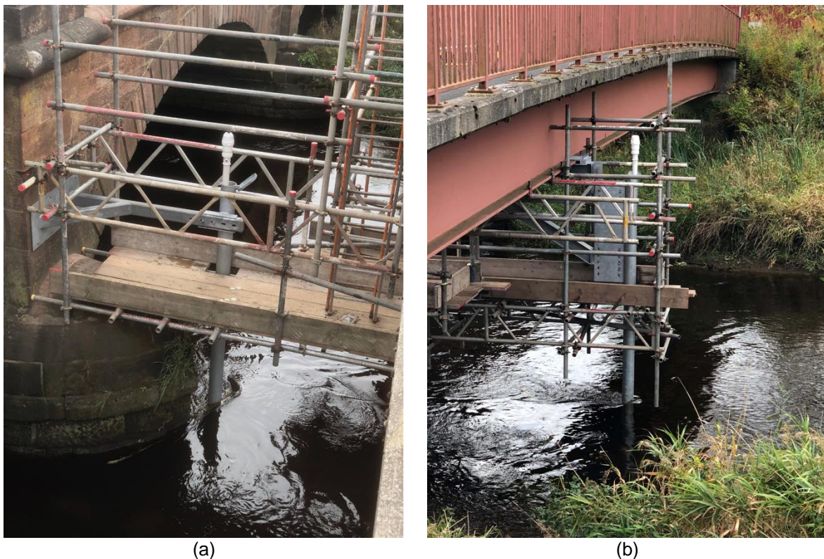
Figure 26. (a) Dielectric probe for total scour at the pier; (b) dielectric probe for degradation and constriction scour [62].
