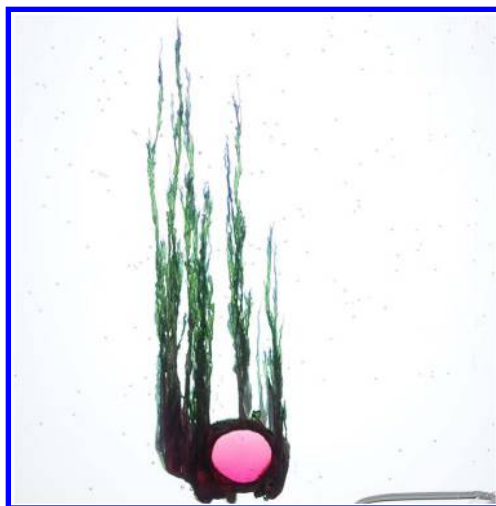
Figure 3. \text{CoCl}_2 pellet reacting with 1.5 M \text{Na}_2\text{SiO}_3 in a 2D experiment in a vertical Hele-Shaw cell shows fluid-flow effects of buoyancy and osmosis.
