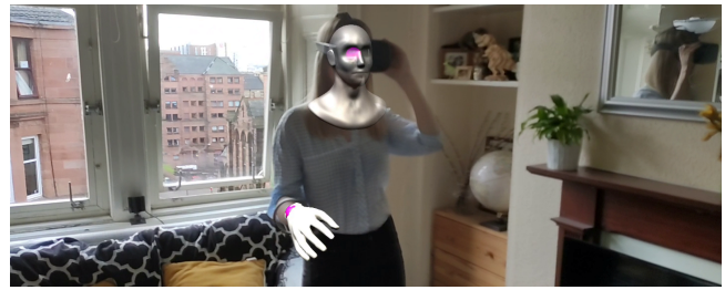
Figure 4: Shows an Oculus Quest and Android ARCore device both aligned using one-point alignment, captured from the perspective of the ARCore smartphone device with pass-through video enabled. The pink spheres represent the center of gravity of the headset and controllers, with a head and hand models attached to those points in the XR player prefab. See video figure for footage this picture was taken from.
