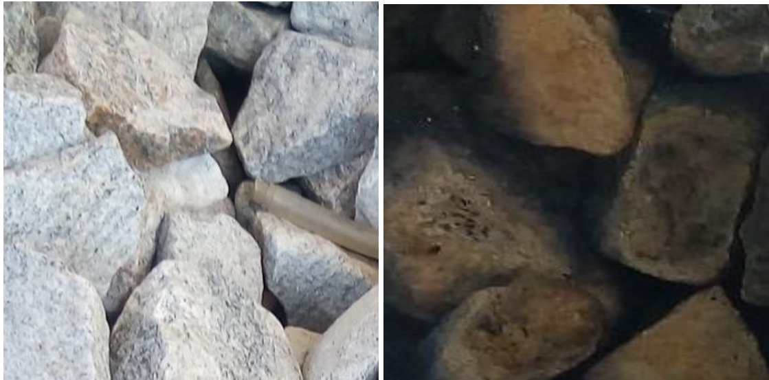
356 Figure 5: Picture of coarse gravel during installation(left/a) and one month after 357 commencement of system operations(right/b).
