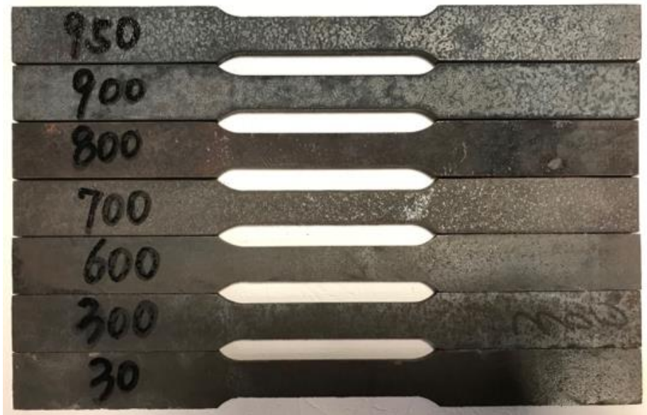
Fig. 4. S690 high strength steel longitudinal coupons at room temperature and after exposure to different levels of elevated temperatures.
