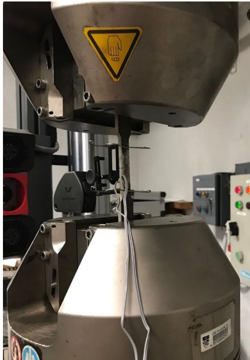
Fig. 5. Tensile coupon test setup.
