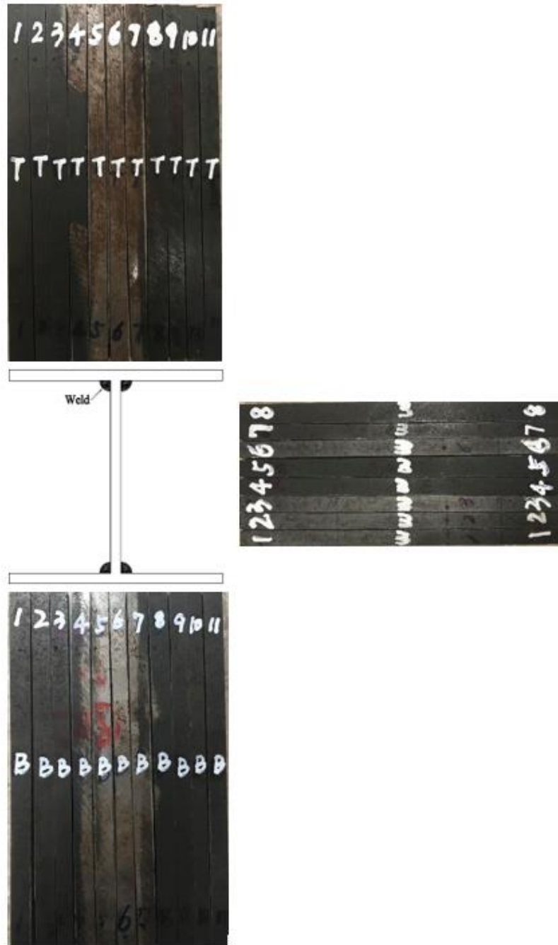
Fig. 10. Typical sectioned S690 high strength steel welded I-section specimen.
