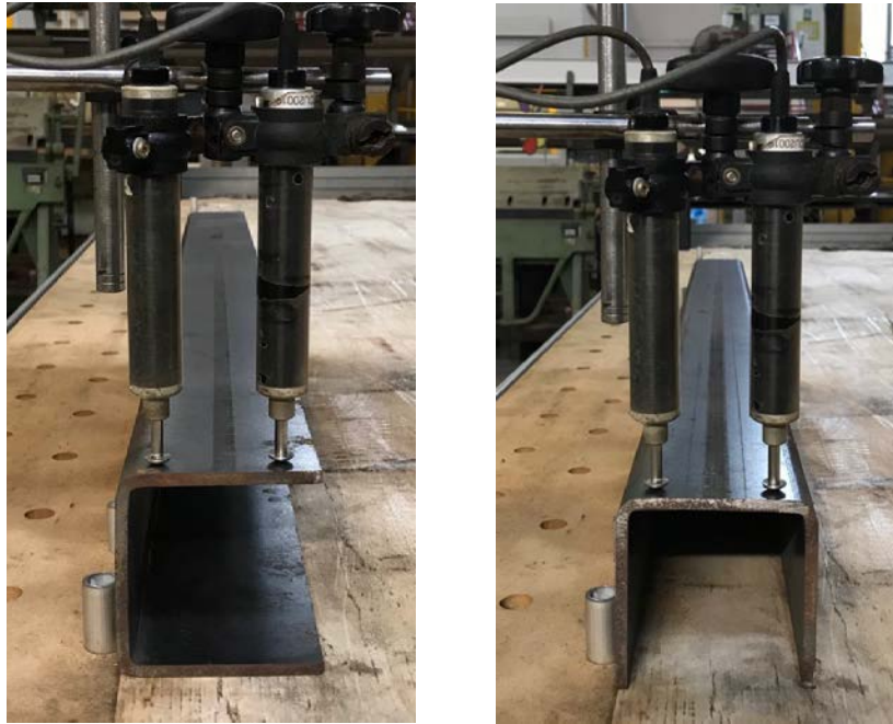
Fig. 4. Test setups for initial local geometric imperfection measurements.
