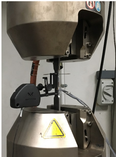
Fig. 2. Tensile coupon test setup.
