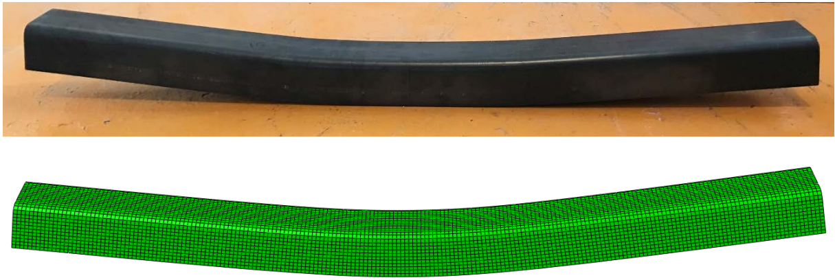
Fig. 8. Experimental and numerical failure modes for press-braked S690 high strength steel channel section beam specimen C 80×60×5-n.
