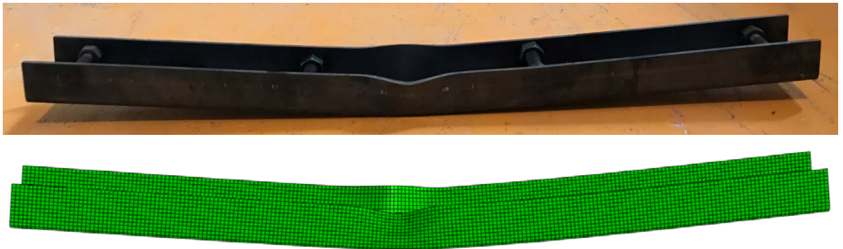
Fig. 9. Experimental and numerical failure modes for press-braked S690 high strength steel channel section beam specimen C 80×60×5-u.
