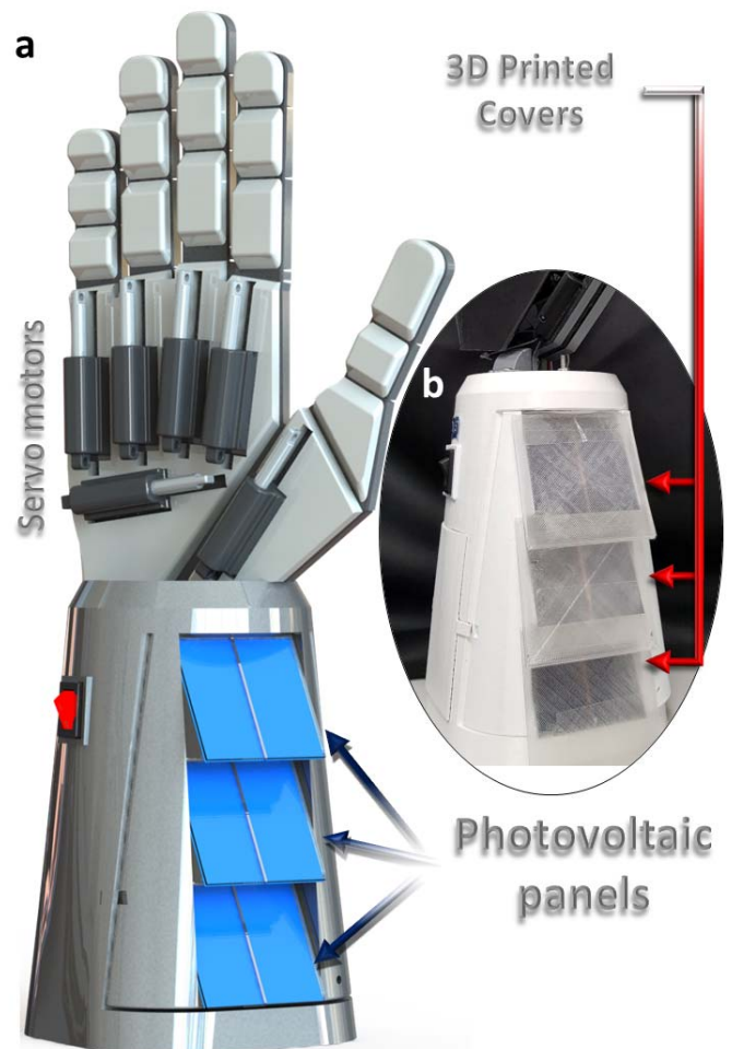
Fig. 1. a) 3D printed robotic hand with three photovoltaic panels. b) 1mm thickness covers attached on the top to reduce wear and tear.
