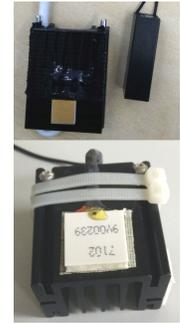
(b) Peltiers and vibrotactile Haptuator
