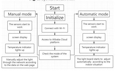
**Fig. 2:** System flowchart VI. SYSTEM ANALYSIS
