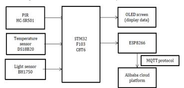
Fig. 1: System Architecture
