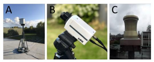
Figure 2. The diversity of observatory infrastructure present in the UK's fireball networks. A) UKFN all sky digital camera. B) UKMON narrow angle CCTV video camera. C) FRIPON all sky video camera.
