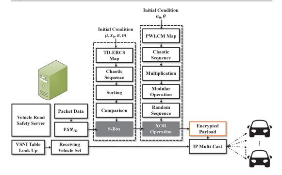
FIGURE 4 Downlink flow diagram
