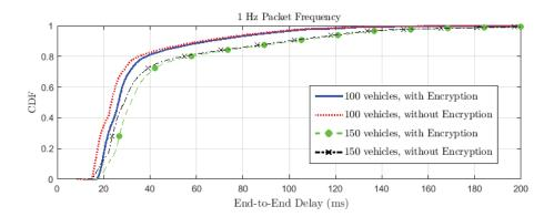
**FIGURE 7** End-to-End delay with 100 and 150 vehicles transmitting vehicle safety messages at 1 Hz packet frequency.
