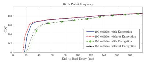
**FIGURE 8** End-to-End delay with 100 and 150 vehicles transmitting vehicle safety messages at 10 Hz packet frequency.
