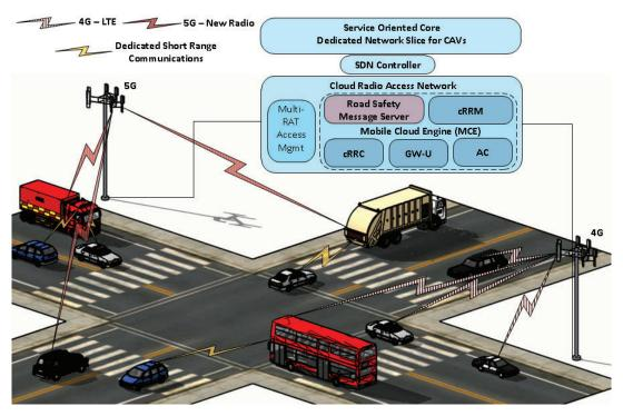
FIGURE 1 5G Communication Network for CAVs.
