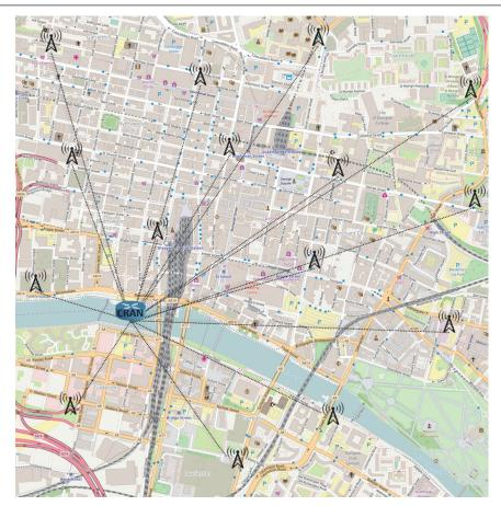
**FIGURE 2** The 2x2 km<sup>2</sup> modelled area of Glasgow City Centre with 14 existing LTE Masts of EE.
