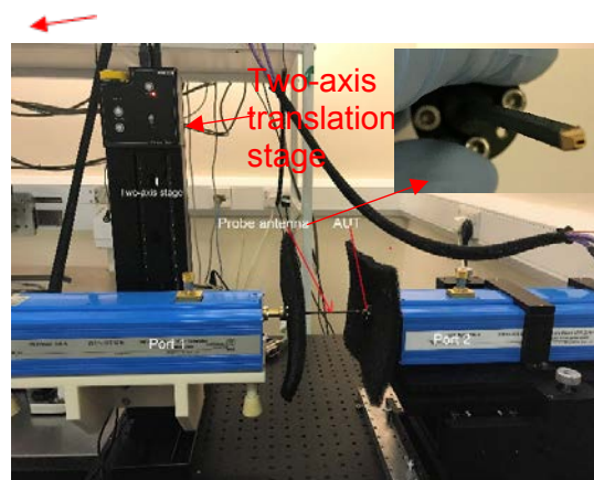
Fig. 1 Measurement setup and the AUT Setup.
