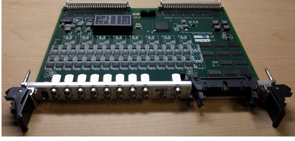
Figure 14: Discriminator Scaler module (DSC2). 16-channel general purpose discriminator and scaler module designed as a 6U VME card.
