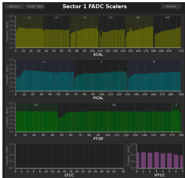
Figure 35: An example of the JLab FADC250 scalers for the CLAS12 PMT-based detector systems.
