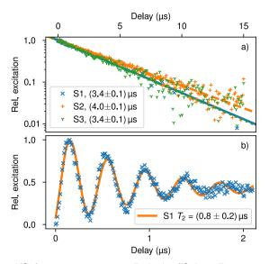
**Fig. 4 Lifetime measurements. a** Excitation lifetimes  $T_1$  measured in samples S1, S2, and S3 range between 3.4 and 4  $\mu$ s. **b** Ramsey fringes measured in S1 yield a dephasing time  $T_2$  of  $(0.8 \pm 0.2) \, \mu$ s.
