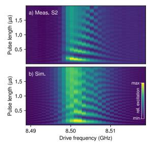
**Fig. 3 Rabi oscillation frequency dependence. a** Rabi oscillations measured in S2 (50 nm long wire) in a span of 30 MHz around the low-power transition frequency of 8.504 GHz. The distinct asymmetry can be attributed to higher level excitations and a relative anharmonicity between 1 and 2 MHz. **b** Result of the numerical Floquet matrix calculation of the density matrix master equation for an anharmonic oscillator with 1.3 MHz anharmonicity. This agrees with an estimation from Fig. 2.
