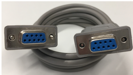
Fig. 2. A serial cable with 9-pin female connectors.
