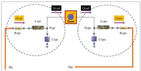
**Fig. 2** Electrical analogue model of the Berlin Heart INCOR pump. Plv ad Pas are the left ventricular and systemic arterial pressures respectively. Input (output) pump cannula is modelled with a resistance Rvpi (Rvpo), a compliance Cvpi (Cvpo) and an inertance Lvpi (Lvpo). Qvad is the pump flow and Qvpi (Qvpo) is the input (output) cannula flow
