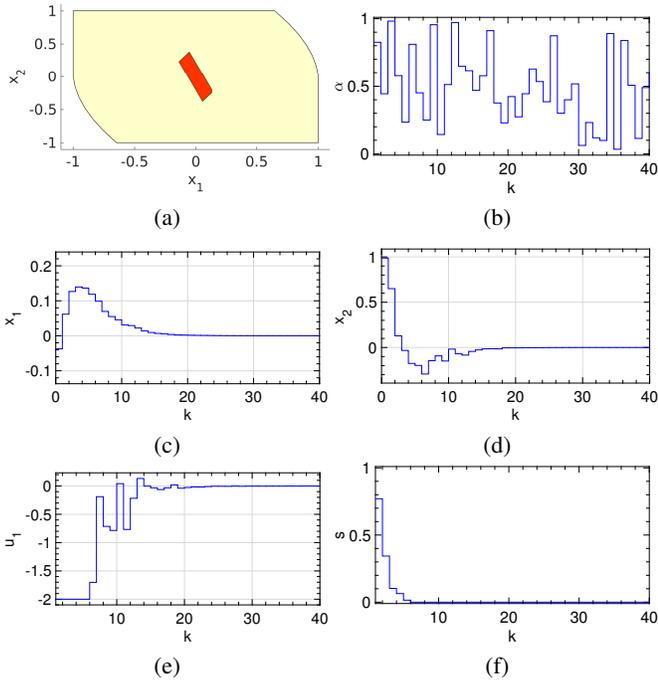
Fig. 2: (a): Invariant sets. The yellow set is the outer  $M$ -step controllable set  $P^{66}$ ; the red set is the MAS for the feedback controller  $u = -Kx$ ; (b):  $\alpha(k)$  realisations; (c), (d), (e): state and control trajectories; (f): Interpolating coefficient for cIC.
