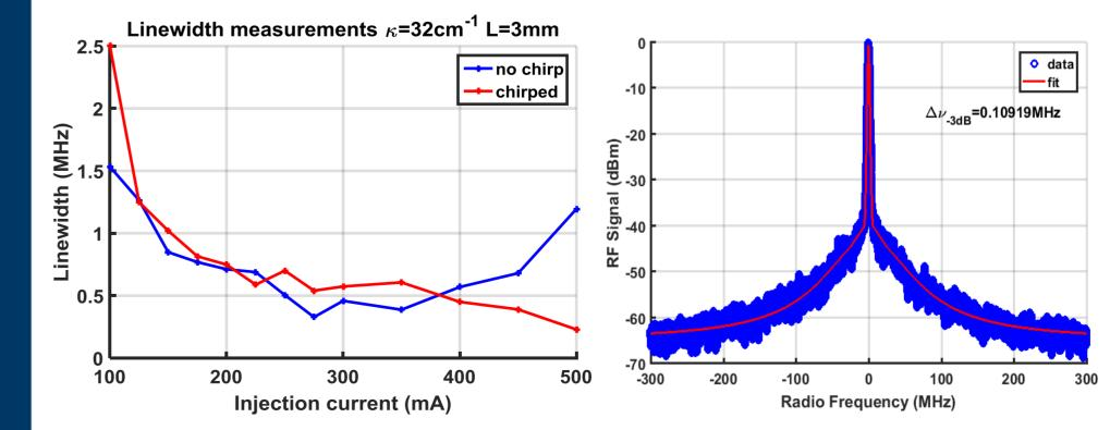
Under the same fabrication conditions narrower linewidth for chirped device, as narrow as 109kHz at high-power operation.
