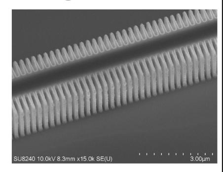
Phase shift layer to solve mode degeneracy and allow single mode operation.
