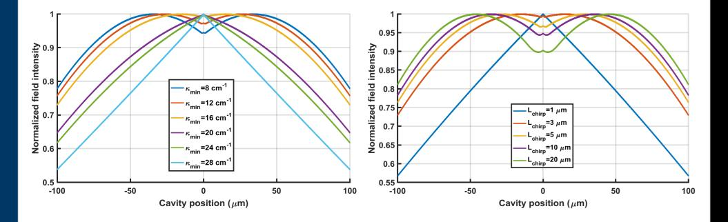
The configuration giving the most uniform distribution, i.e. closer to no phase shift grating, is the best for the narrow linewidth at high-power.
