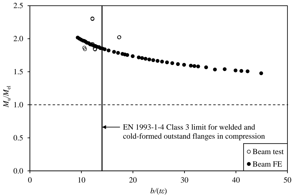
Fig. 14. EC3 Class 3 limit for stainless steel equal-leg angles in geometric axis bending.
