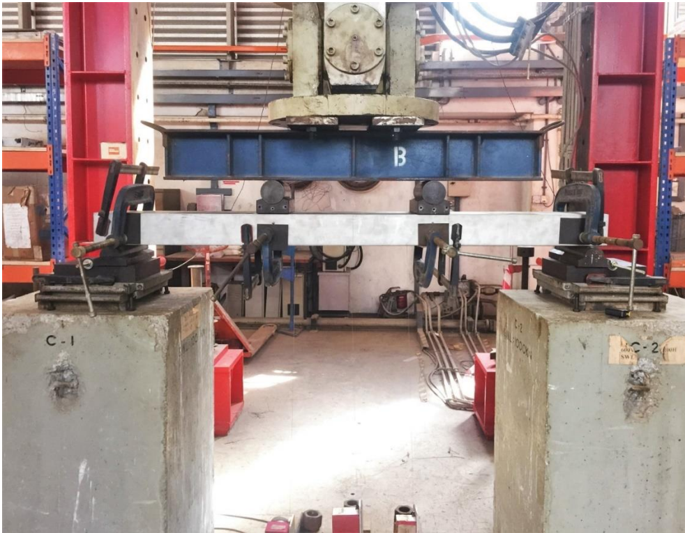
Fig. 8. Test rig for laterally restrained double-angle beams bent about the geometric axes in the ‘reverse L’ orientation.
