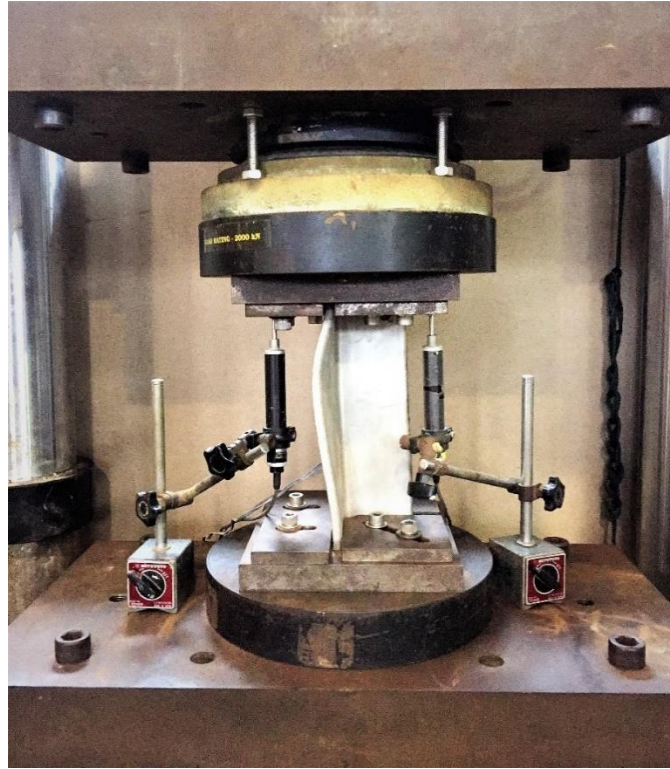
Fig. 3. Equal-leg angle stub column test rig.
