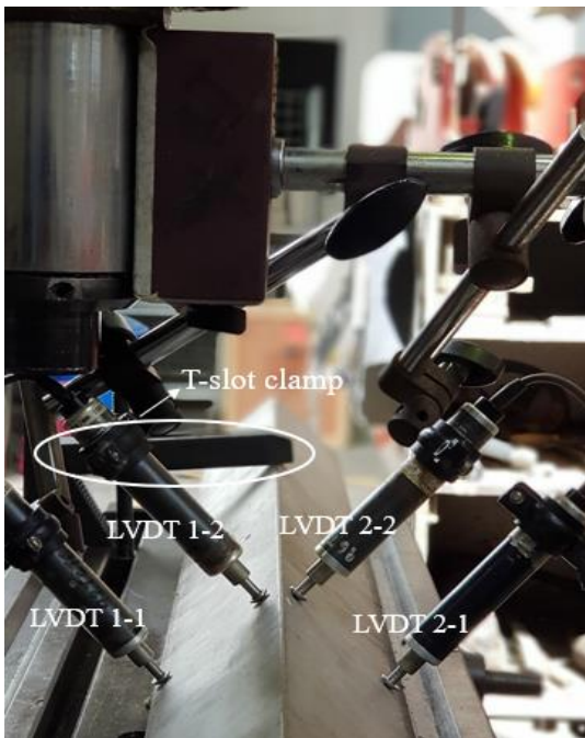
(c) Rig for local geometric imperfection measurements.
