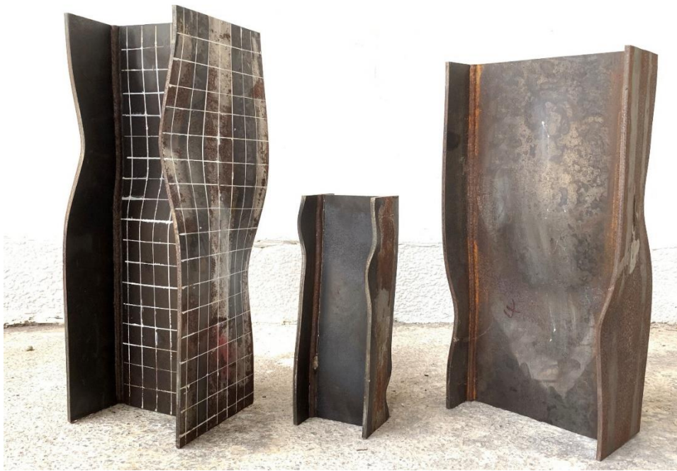
Fig. 13. Failure modes of S690 welded I-section stub column specimens (from left to right: I-150×150×5-1, I-90×70×5-1, I-200×100×5-1).
