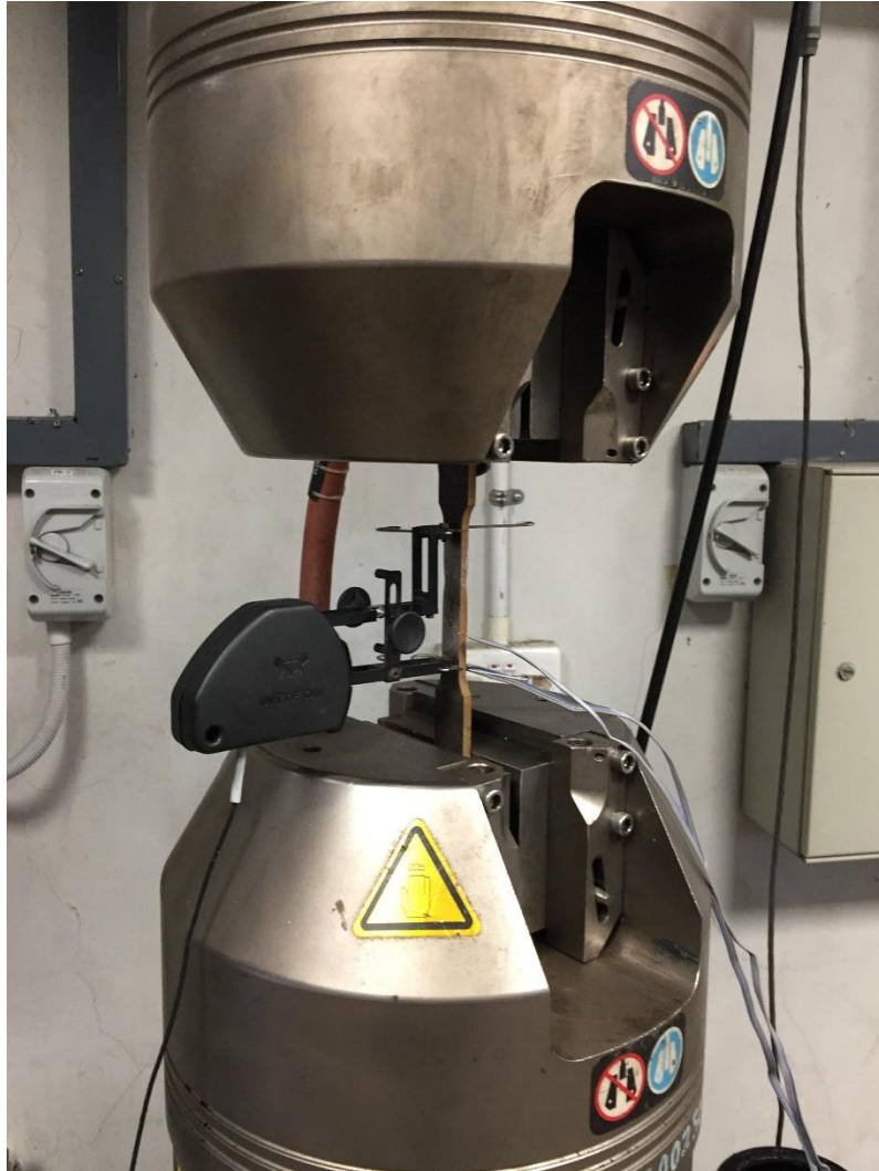
Fig. 1. Tensile coupon test setup.
