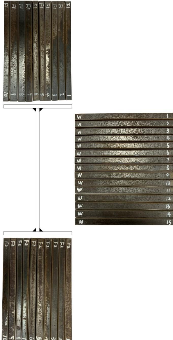
Fig. 5. Typical sectioned S690 welded I-section I-200×100×5.
