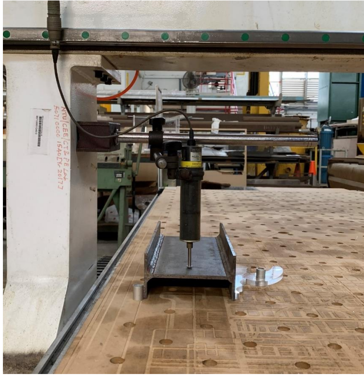
Fig. 9. Test rig for initial local geometric imperfection measurements.
