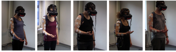
Figure 7: Although only the biceps and not the muscle required for rotating hands to face upwards were actuated, participants rotated their hands when their virtual faced upwards. This suggests that EMS-based feedback must not necessarily actuate the entire movement. Instead, EMS can partially actuate movements, while visual feedback nudges users to subconsciously complete the entire movement.
