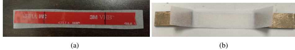
Figure 1: Specimen preparation. (a) Step 1: VHB tape with a required length is attached to a clean silicon paper, (b) Step 2: after removal of the red protective surface of VHB
