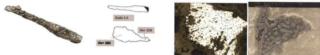
FIGURE 5. LB22 A1980.552 TOOL (CHISEL) DISPLAYING SUBSTANTIAL HARDNESS WHICH DERIVES, EITHER FROM AN ELEVATED PHOSPHORUS CONTENT WITHIN THE FERRITE MATRIX AND/OR CEMENTITE. BOTH PHOSPHORUS AND CARBON WERE AT THE TIME OF THE ANALYSIS, AND WITH THE INSTRUMENTATION USED, NOT POSSIBLE TO DETECT. FROM LEFT TO RIGHT: OBJECT; PLACE OF SECTION REMOVED; MICRO-HARDNESS MEASUREMENTS AT TWO DIFFERENT SPOTS ON THE SECTION; IMAGE OF SECTION (FERRITE=BRIGHT PHASE; CORROSION AREAS = DARK PHASE); SLAG INCLUSION SHOWING GLOBULAR WUSTITE IN A PHOSPHORUS RICH GLASSY MATRIX; AREA SURROUNDING THE SLAG INCLUSION IS THE METAL.
