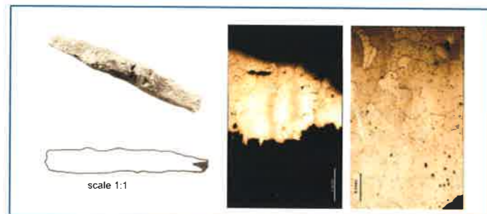
FIGURE 3. LB20. A1980.612 THIS IS FERRITE WITH SMALL AMOUNTS OF CARBIDES OR NITRIDES TO ACCOUNT FOR THE REGISTERED HARDNESS OF HV=141 OR 125. TOOLS MADE EXCLUSIVELY OF FERRITE WOULD BE TOO SOFT TO USE AND SO UNDESIRABLE.
