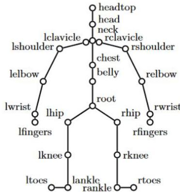
**Fig. 1.** Skeletal Kinematic chain model consisting of rigid bones that are flexibly connected by joints, which are highlighted by circular markers and labelled with joint names [15].
