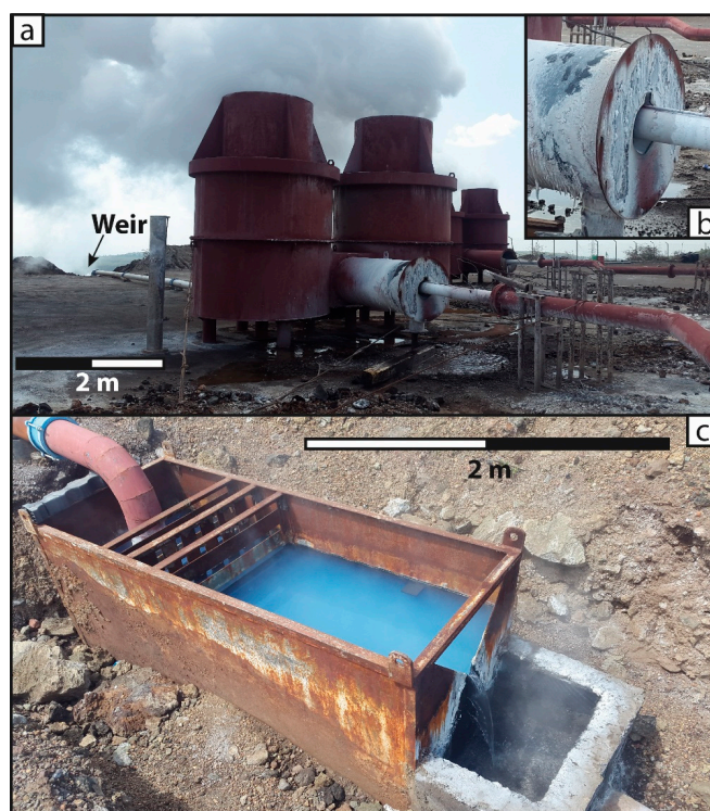
Figure 4. Menengai production test well infrastructure. (a) MW-17a (UTM 0171344, 9976440) flashing silencer and steam release chambers showing the weir sampling location. (b) Close-up of MW-17a silencer entry demonstrating significant silica precipitation. (c) Weir outlet and sampling location for MW-09 (UTM 0172910, 9976964). All images taken by N.M.B.
