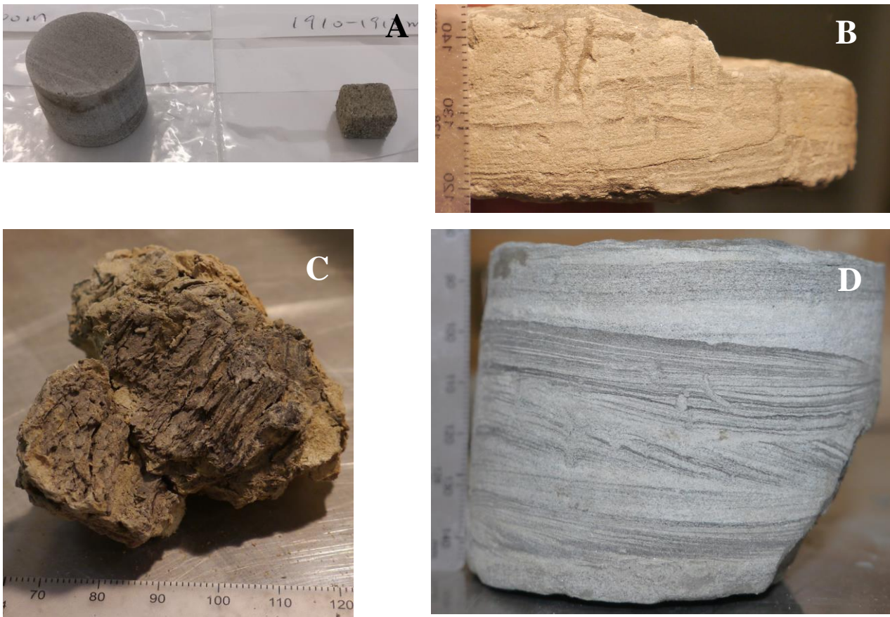
Figure 2: (A) Core samples from the nearby Kondoros-1 (Kond-1) well (Figure 1) from 1500-1900 m depth, prepared for XCT porosity scanning and flow through experiments. (B) fine laminated sandstone core sample with rootlets interrupting ripple structures from Gyoma-1 well at 1990-1995 m depth. (C) light grey to green Marl and grey silt laminations in an unconsolidated core fragment from Kond-1 well at some 1500 m depth. (D) thin light grey laminated sandstone with small burrows intersecting dark grey lignite-rich laminations.
