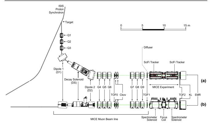
Fig. 2 a Top and b side views of the MICE Muon Beam line, its instrumentation, and the experimental configuration. A titanium target dipped into the ISIS proton synchrotron and the resultant spill of particles was captured with a quadrupole triplet (Q1-3) and transported
