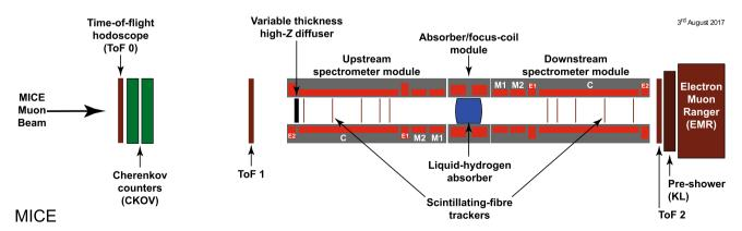
**Fig. 1** Schematic diagram of the MICE experiment. The red rectangles represent the coils of the spectrometer solenoids and focus-coil module. The individual coils of the spectrometer solenoids are labelled E1, C, E2, M1 and M2. The various detectors (time-of-flight hodoscopes
