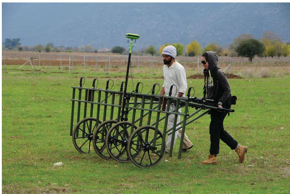
Figure 1. SENSYS Magnetometer MX in use at Mantinea. The device is equipped with a GPS rover station that communicates with a dGPS base station.
