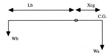
The aircraft is brought to a level position by adding a weight ballast  $W_b$  at a length  $L_b$  from the reference point. The point at which the aircraft weight  $W_a$  is applied (i.e. the c.g. position), is denoted by  $X_{cg}$  and is calculated by taking the moment equation about the reference point:
