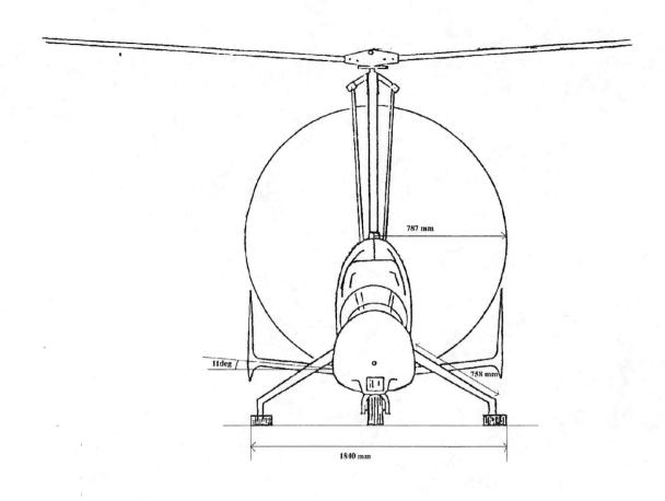
Figure 1 Frontal view of gyroplane
