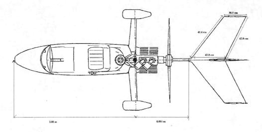
Figure 2 Planar view of gyroplane
