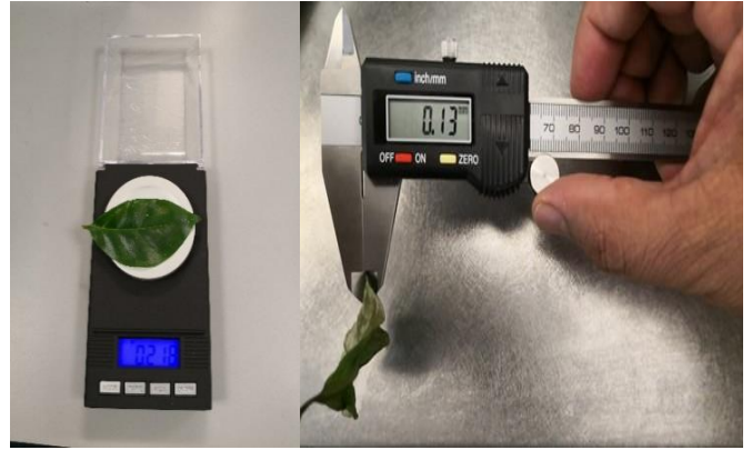
Figure 3. Demonstration of measuring the weight and thickness of leaf using Digital Scale and Vernier Calliper.
