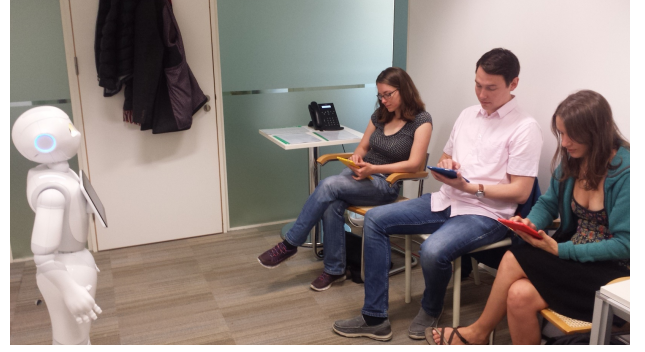
Figure 2: Experimental Setting. The observers sit at a distance of roughly 1.5 meters from the robot and fill out the questionnaires using a tablet.
