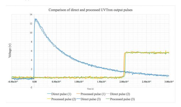
**Figure 2.** Comparison of the direct pulse recorded directly from the UVTRON and the processed pulse generated by the driver circuit (C10807, Hamamatsu) during normal UVC detection operation. The two pulses generated for three separate photon events (1, 2, 3) are shown.
