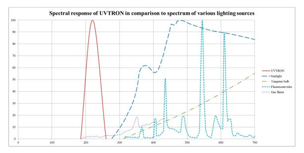
Figure 1. Spectral response of the R9533 UVTRON. Derived from data from Hamamatsu [7] and OSRAM [8].
