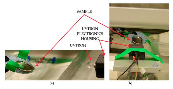
**Figure 4.** Showing the set up at the National Nuclear Laboratory (**a**) view from the side showing the vertical alignment of the UVTRON and source, and (**b**) showing the horizontal alignment of the UVTRON to the source.
