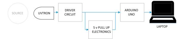
Figure 3. Block diagram of the set up used in these experiments.
