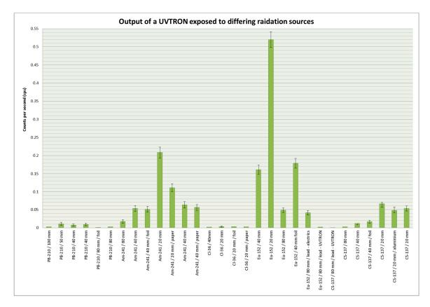
**Figure 6.** Results of the experiments carried out at Lancaster University. The error bars shown are the confidence interval as included in Table 3. Where no error bar is shown, this is due to the count being below the threshold to calculate the confidence interval, i.e., less than the limit of detection as laid out by Hurtgen et al. [10].
