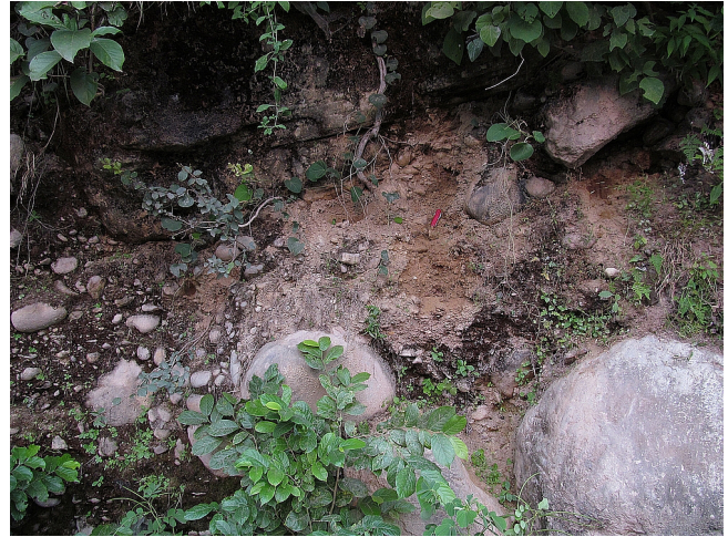
Figure A15. RLB – \sim 42 m above modern channel on roadside cut. Poorly sorted, structureless fluvial conglomerate. Large, rounded boulders, cobbles and sands (Ray and Srivastava, 2010); 90 mm long penknife for scale.
