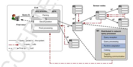
' igure 1: Query processing mechanism with the introduction of TinyOS.
