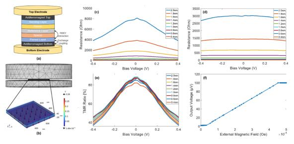
Fig.1 Schematic of the TMR stack layout used for FEM simulations.
