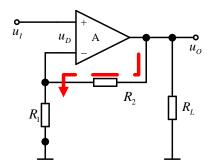
Fig. 4. "Voltage feedback" that feeds back the output voltage portion
