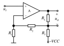
Fig. 5. "Current feedback" that feeds back the output current portion
