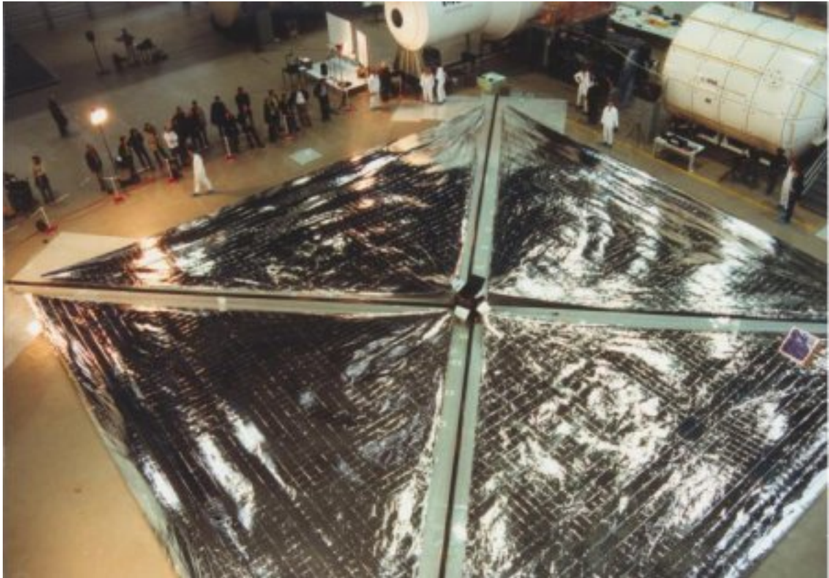
Figure 1 – Ground deployment test of a (20 m) 2 sail, DLR Cologne, in the EAC hall (note space station practice modules in the background) December 17 th , 1999
