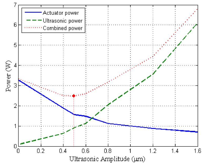
Power. In addition to reducing the required overhead force, ultrasonics can also reduce the total power consumption. An optimum level of vibration can be found which balances the power consumption saved by the actuator, with the additional power consumed required by the ultrasonic transducer.
