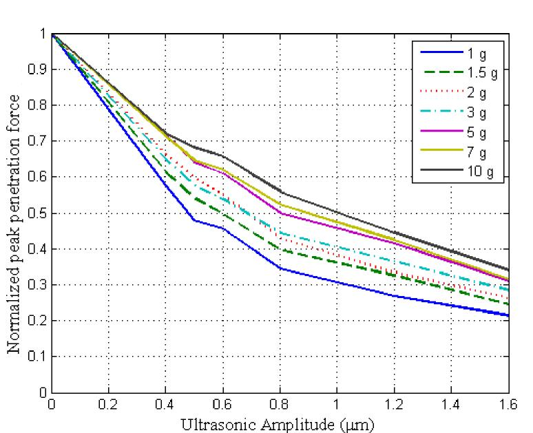
that ultrasonics in higher gravities are less effective at reducing penetration force. Extrapolating this result signifies that ultrasonics could have an even greater impact in low gravity environments, and could potentially be used to great effect in lander missions.
