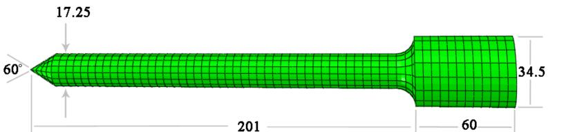
**Penetrator.** A titanium probe (above) was designed to vibrate at 20 kHz, with a Langevin transducer providing excitation amplitudes from 0.4 to 10 μm.
