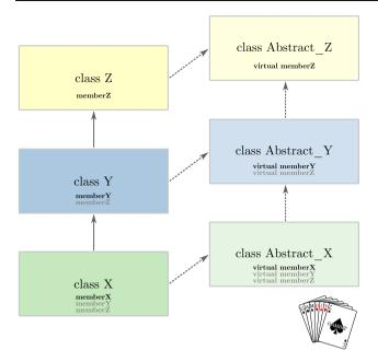
**Fig. 3** The basic class 'ladder' pattern generated by BOSS in order to allow runtime loading of classes X, Y and Z, where Z is the parent of Y, which is in turn the parent of X. The original class hierarchy is mirrored by the abstract parent classes generated by BOSS. Virtual inheritance, illustrated here by dashed arrows, is used to avoid ambiguities. Member functions in the original classes are matched by pure virtual member functions in the abstract classes
