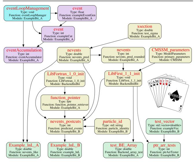
Fig. 5 An example dependency tree generated in the initialisation stage of a GAMBIT scan. Each block corresponds to a single module function, with the red text indicating its capability. Arrows indicate resolution of dependencies of different module functions with the results of others. The functions selected by the dependency resolver to provide the observables and likelihoods requested in the Obslikes section of the scan's input YAML file are shaded in green. Module
