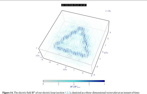
**Figure 14.** The electric field E<sup>a</sup> of our electric foop (section 3.2.2), depicted as a three-dimensional vector plot at an instant of each blue arrow represents an electric field vector, colour-coded and scaled by magnitude.
