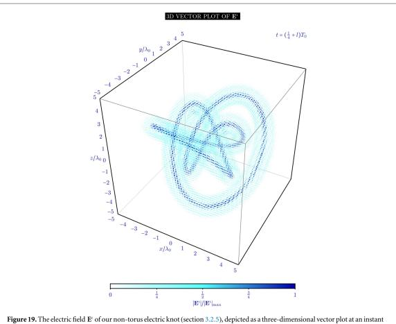
**Figure 19.** The electric held **E**' of our non-torus electric knot (section 3.2.5), depicted as a three-dimensional vector plot at an instant of time: each blue arrow represents an electric field vector, colour-coded and scaled by magnitude. Each of the electric rings comprising the knot has been plotted for  $|s_n| \leq \lambda_0$  and  $|z_n| \leq \lambda_0$  only, for the sake of clarity and to render the task numerically tractable.
