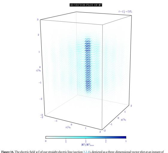
**Figure 16.** The electric field  $\mathbf{E}^{\ddagger}$  of our straight electric line (section 3.2.4), depicted as a three-dimensional vector plot at an instant of time: each blue arrow represents an electric field vector, colour-coded and scaled by magnitude.
