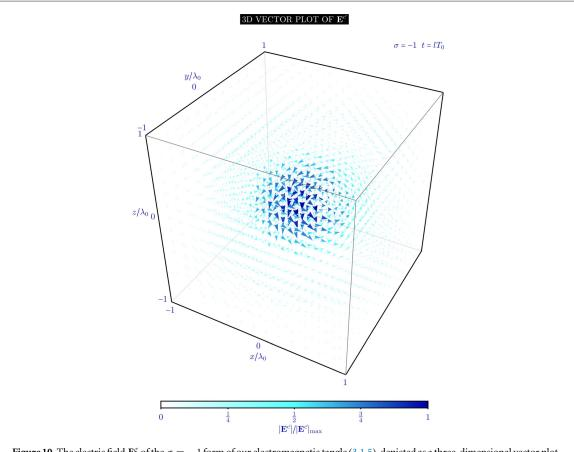
**Figure 10.** The electric field  $\mathbf{E}^{c}$  of the  $\sigma = -1$  form of our electromagnetic tangle (3.1.5), depicted as a three-dimensional vector plot at an instant of time: each blue arrow represents an electric field vector, colour-coded and scaled by magnitude.
