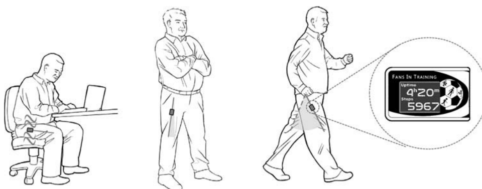
FIGURE 1 —The pocket-worn SitFIT device during sitting, standing and stepping activities. The SitFIT tracks the orientation of the upper thigh, so changes orientation when posture changes from sitting to upright. The display provides real-time feedback of sitting (or upright) time and of step count.
