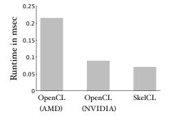
Fig. 5. Performance results for Sobel edge detection
