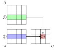
**Fig. 3.** The allpairs computation: Element  $c_{2,3}$  (3) is computed by combining the second row of A (1) with the third row of B (2) using the binary operator  $\oplus$
