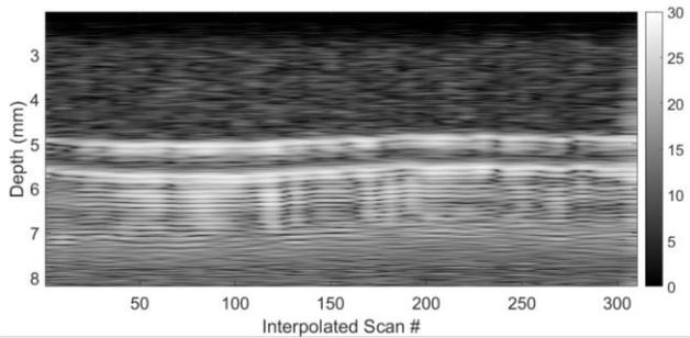
Fig. 5 Porcine small bowel tissue scan *in vivo* obtained with a 30 MHz PVDF transducer physically focused at 6 mm. Scan was obtained via a 12 cm pullback through the small bowel accessed via a surgically inserted stoma.
