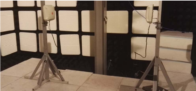
Fig. 6 Radiated test setup in an anechoic chamber.
