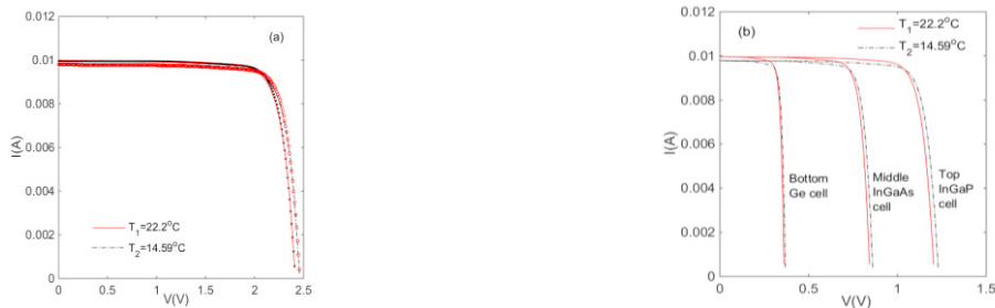
Fig.6 Comparison of (a) measured and (b) model current-voltage I-V curves for the three sub-cells.
