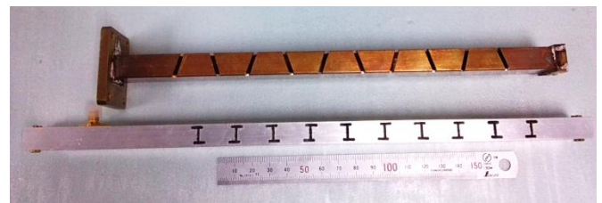
Figure 15: A conventional copper WR-90 inclined edge slot antenna and a Z-slot aluminium tubing antenna.
