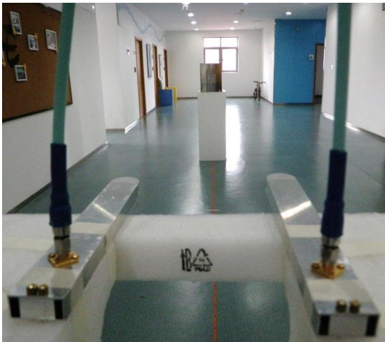
Figure 7: Photograph of bistatic (quasi-monostatic) ranging radar measurement in a 17 m corridor section; end fire antennas in foreground, aluminium plate target at 5 m, corridor end wall with window at 17 m.
