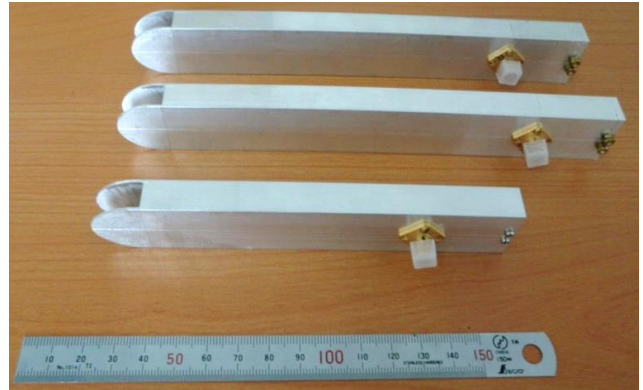
Figure 3: Photographs of prototype end fire antennas; half ellipse length was 18.5mm long on all 3 antennas.
