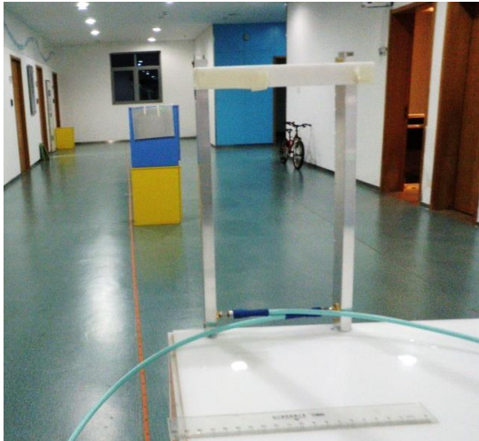
Figure 12: Photograph of bistatic (quasi-monostatic) ranging radar measurement in a 17 m corridor section; inclined-slot 10-slot slotted waveguide antennas in foreground, aluminium plate target at 5 m, corridor end wall with window at 17 m.
