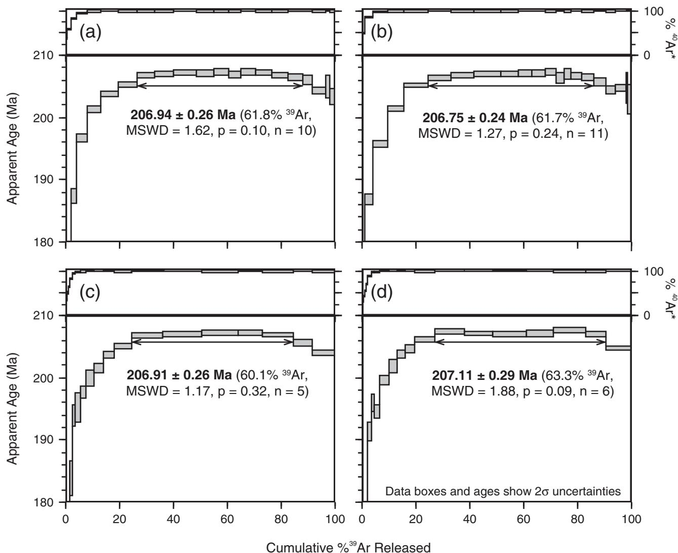
Fig. 3. a–d)  $^{40}\text{Ar}/^{39}\text{Ar}$  incremental-heating analyses of the Babaudus impact melt. The results are highly reproducible between the four aliquots, giving high  $\%^{40}\text{Ar}^*$  yields and plateau ages representing  $>60\%$  of the  $^{39}\text{Ar}$  released. Low-temperature steps yielded younger ages, consistent with the  $<10\%$  smectite clay found in this impact melt sample.
