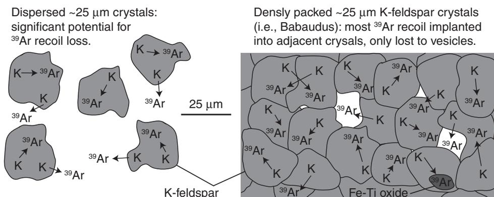
Fig. 5. Schematic diagram demonstrating why, despite the 25 μm mean crystal size, <sup>39</sup>Ar recoil is largely mitigated in the Babaudus sample (right image), due to the closely packed interlocking network of crystals. Voids are white, K-feldspar crystals are mid-gray, and Fe-Ti oxides are dark gray.
