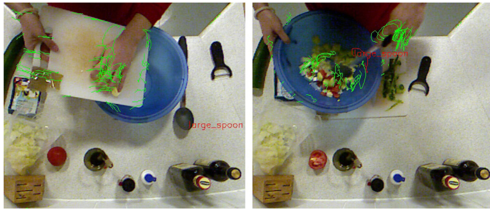
Fig. 3. Point trajectories (green) in the left and right image have similar shape (best viewed in color). However, relative to the trajectory of the large spoon (red), points in the left image move towards whereas most points in the right image move away from this reference trajectory. (For interpretation of the references to color in this figure legend, the reader is referred to the web version of this article.)
